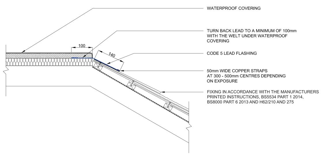
LAY CODE 5 x 240 GIRTH FLASHING OVER TOP COURSE OF SLATE AND ONTO FLAT ROOF. AS DETAIL.
